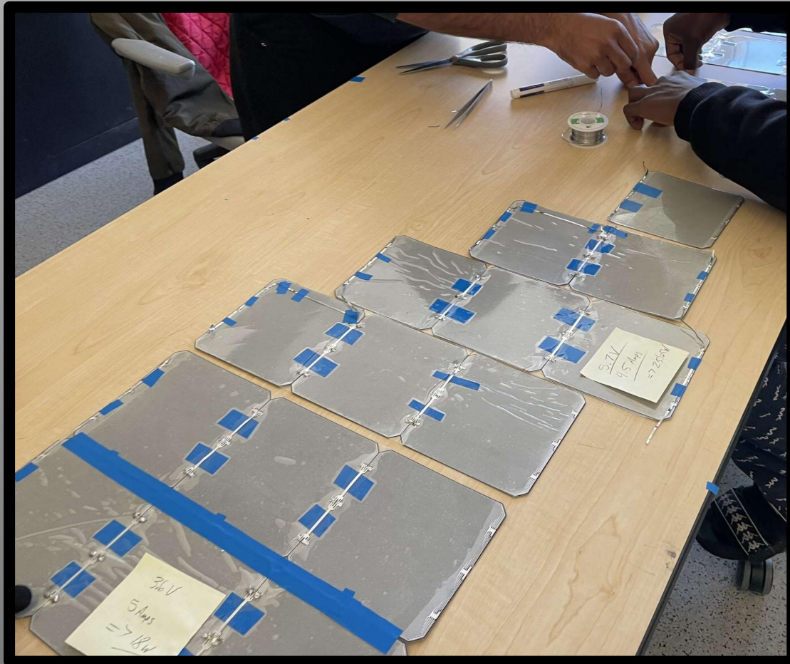
Figure 3: Solar Encapsulation Process (Backside)
